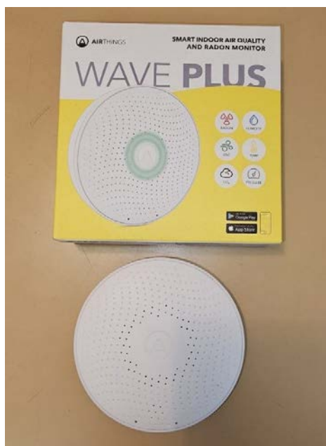
Fig. 1 – Airthings Wave Plus indoor air quality sensor used for the measurements Source: own photographic documentation
