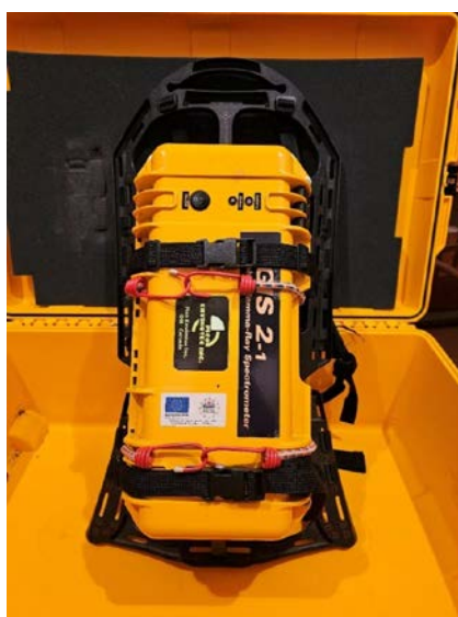
Fig. 2 – PicoEnvirotec PGIS2-1 field gamma spectrometer used for the in situ measurement of natural radioactivity Source: own photographic documentation
