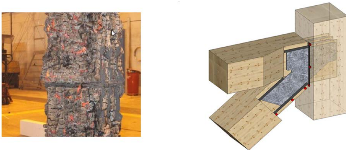
Figure 8 - View of the fire test of the sample with activated fire strips, on the left and the placement of the strips in the slots between the beam, the column and the connecting elements, on the right [10]
